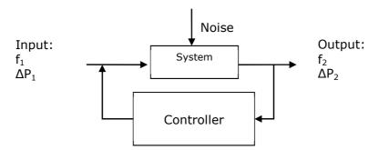
Figure 4: The imbalance management system as a controller
