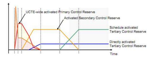
Figure 2: Sequential activation of the different control reserves after a disturbance (UCTE handbook P1 – Policy 1: Load-Frequency Control and Performance [C]).
