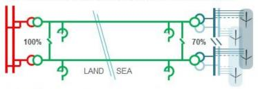
OPTION 4: full coupling (on+offshore coupling)
