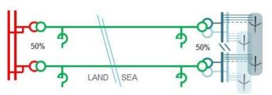
OPTION 2: basic coupling (coupling offshore at 66kV/33kV side)
