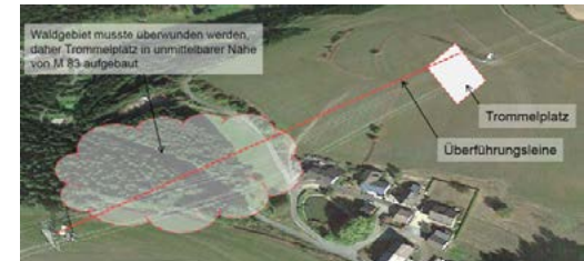
2. Vehicle moves, pulls transfer line, which rotated the drum.
