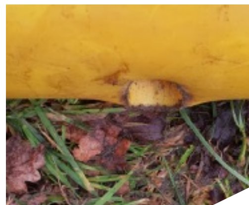
Punctured gas pressure main
