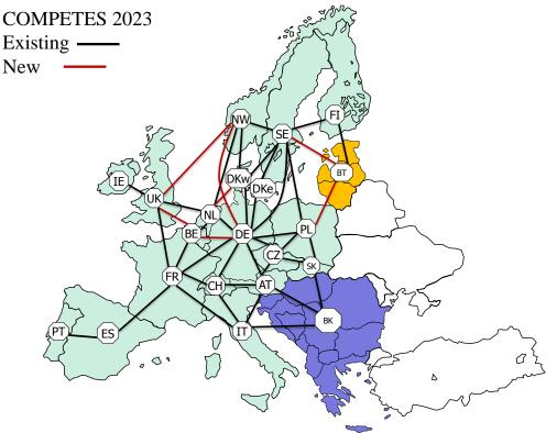
**Figure 24** Geographical coverage in COMPETES UC and the representation of the cross-border transmission links in 2023 according to Ten-Year Network Development Plans of ENTSO-E
