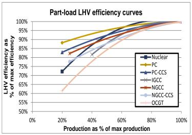
Figure 25 Part-load efficiency curves for different technologies. Source: ECN (Brouwer et al. (2013))
