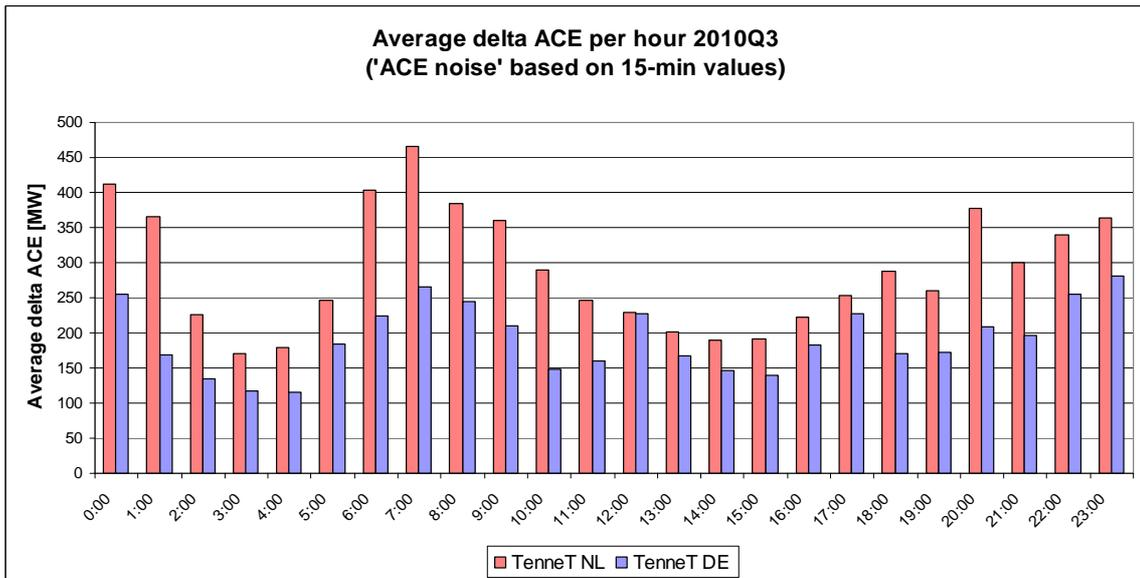
**Figure 28 Average Delta area control error per hour in Q3**
