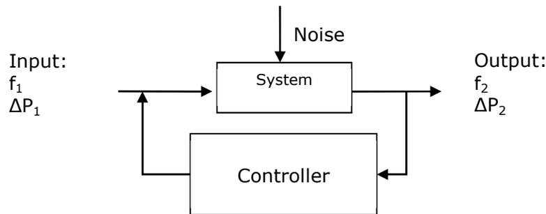
**Figure 4: The imbalance management system as a controller**
