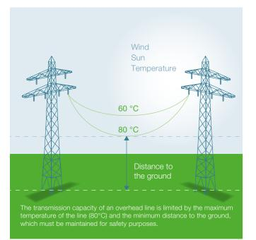
Using these meteorological data the network control centre calculates real-time the dynamic loadability of the high-voltage line. The calculated extra transmission capacity can then be used.
