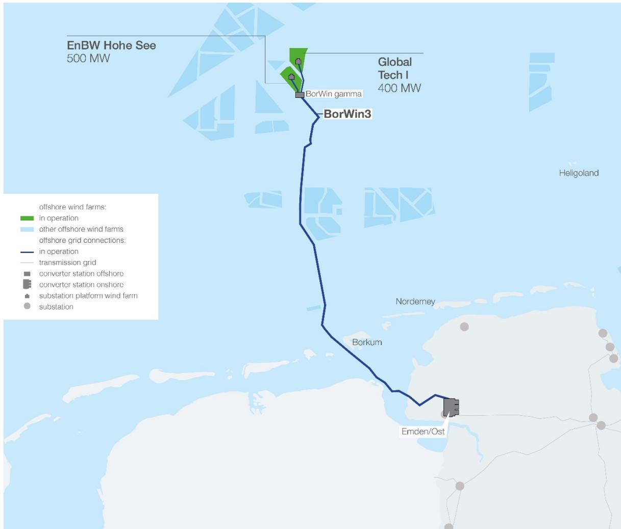
*Image caption: Schematic route of the offshore grid connection project BorWin3*
