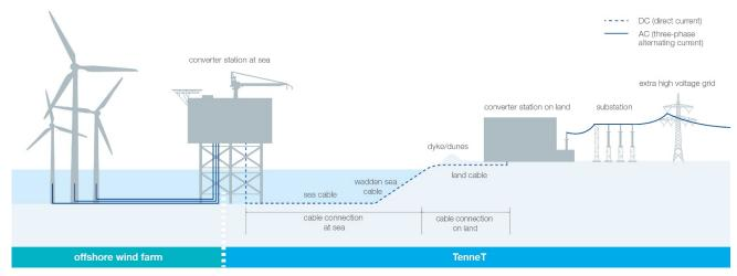
With the innovative 66 kV connection, the wind farms are directly connected to TenneT's offshore platform. Transformer stations in the offshore wind farms are thus no longer necessary..
